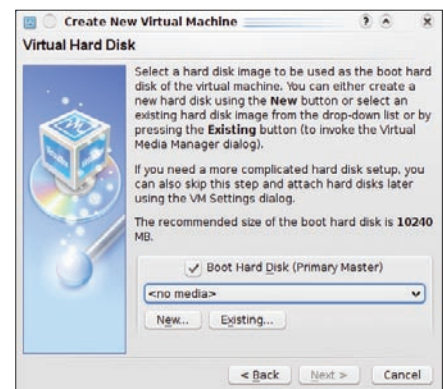
Figure 5: Unless you defined a previous virtual disk, you'll need to create one. Because it is possible to reuse disk images, previous images will be listed here.
