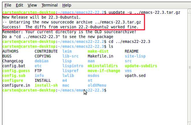
Figure 2: The uupdate command unpacks a source code archive and creates a debian subdirectory based on the content of the existing package.
